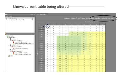
Most maps from Dynojet will include a base Target AFR table. These settings are intended to deliver optimal performance while still maintaining decent fuel mileage in the cruise area (for most models).
