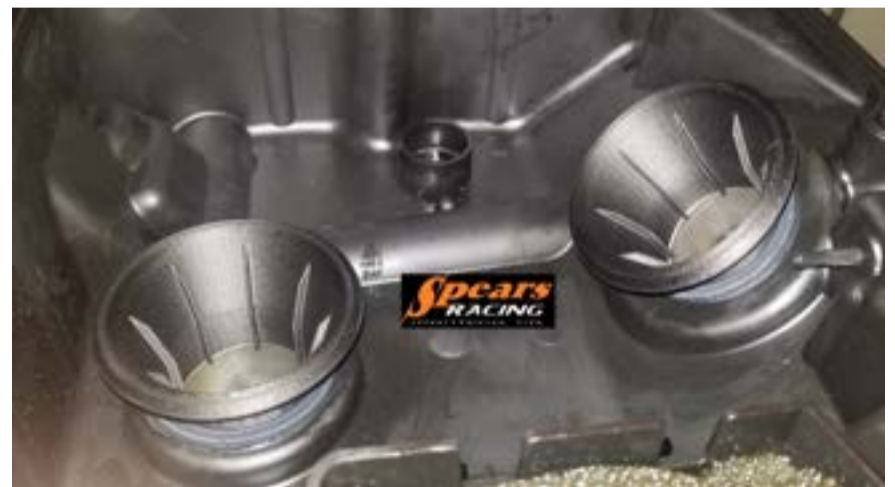
Figure 1: New manifold alignment tabs mated with the airbox alignment tabs.
