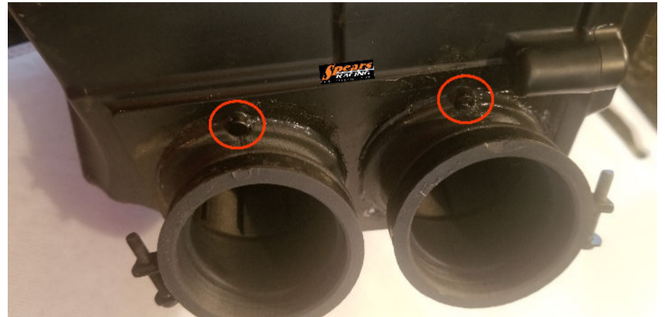
Figure 2: New manifold alignment tabs mated with the airbox alignment tabs.
