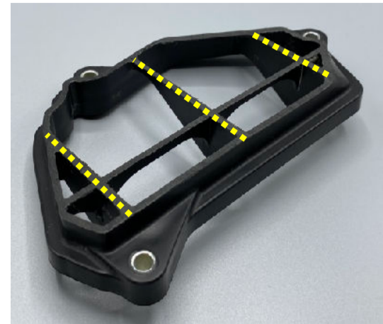
Figure 2: Air filter cover hold-down ribs exposed after cutting.
