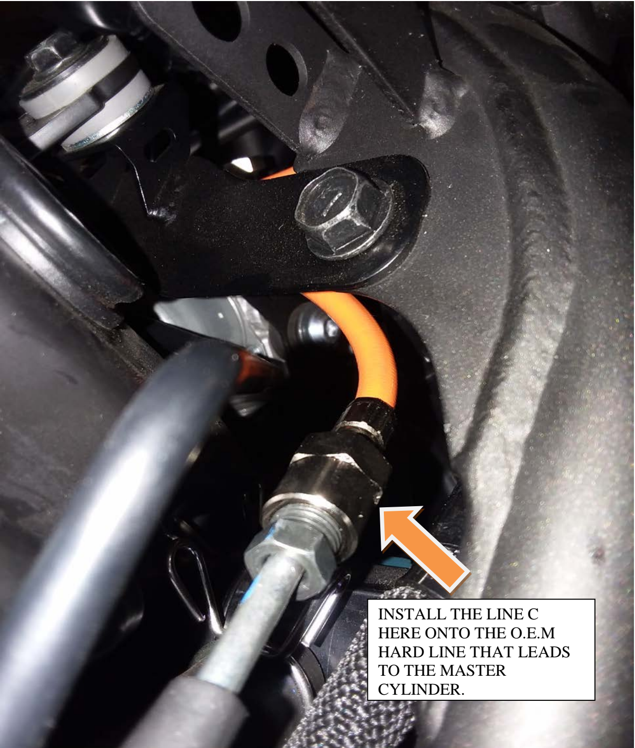
FIGURE 6 CONTINUED: HARD LINE INSTALLATION
