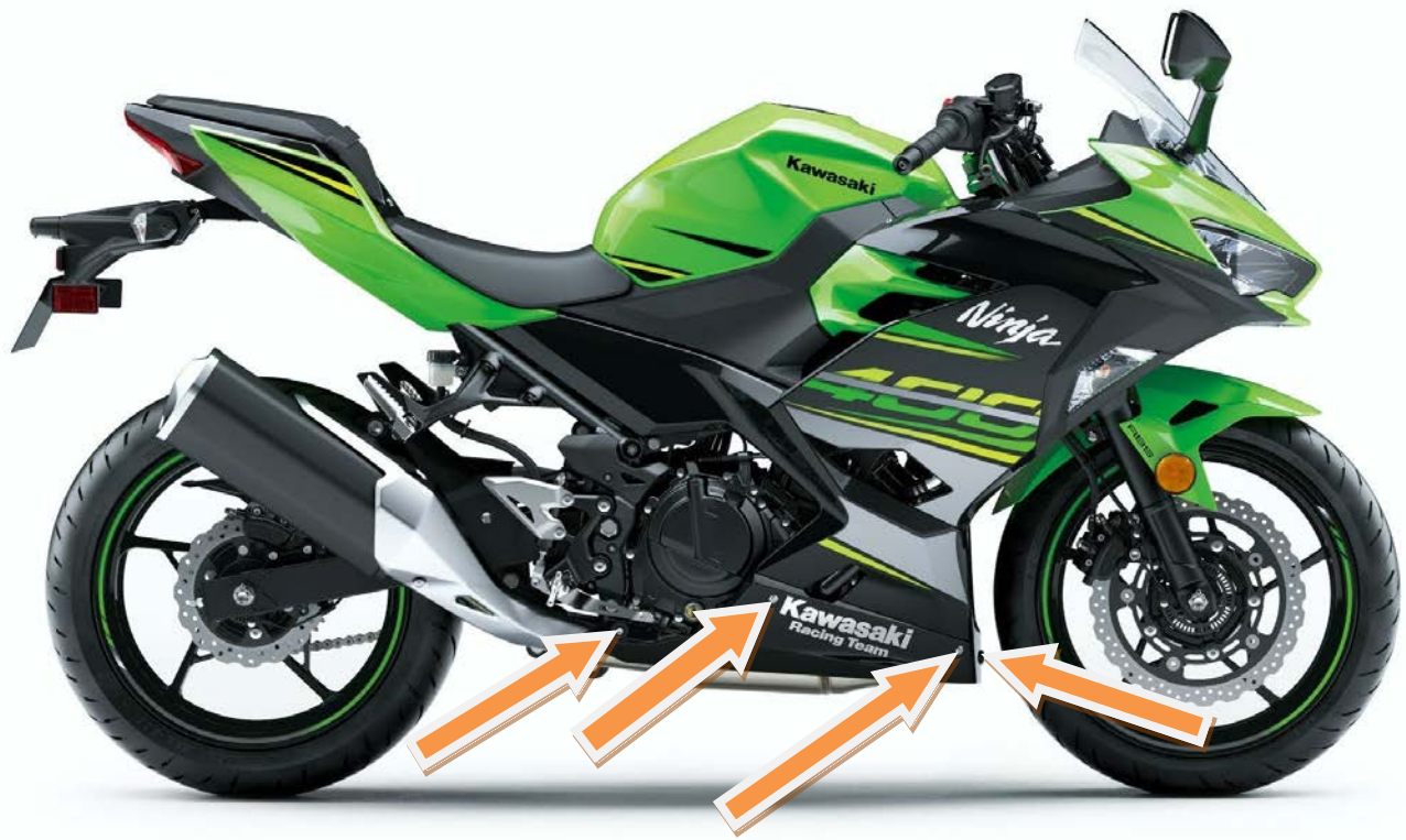
FIGURE 2 CONTINUED: WHERE EVER THERE IS AN ARROW THERE IS A PUSH PIN OR BOLT THAT MUST BE REMOVED
