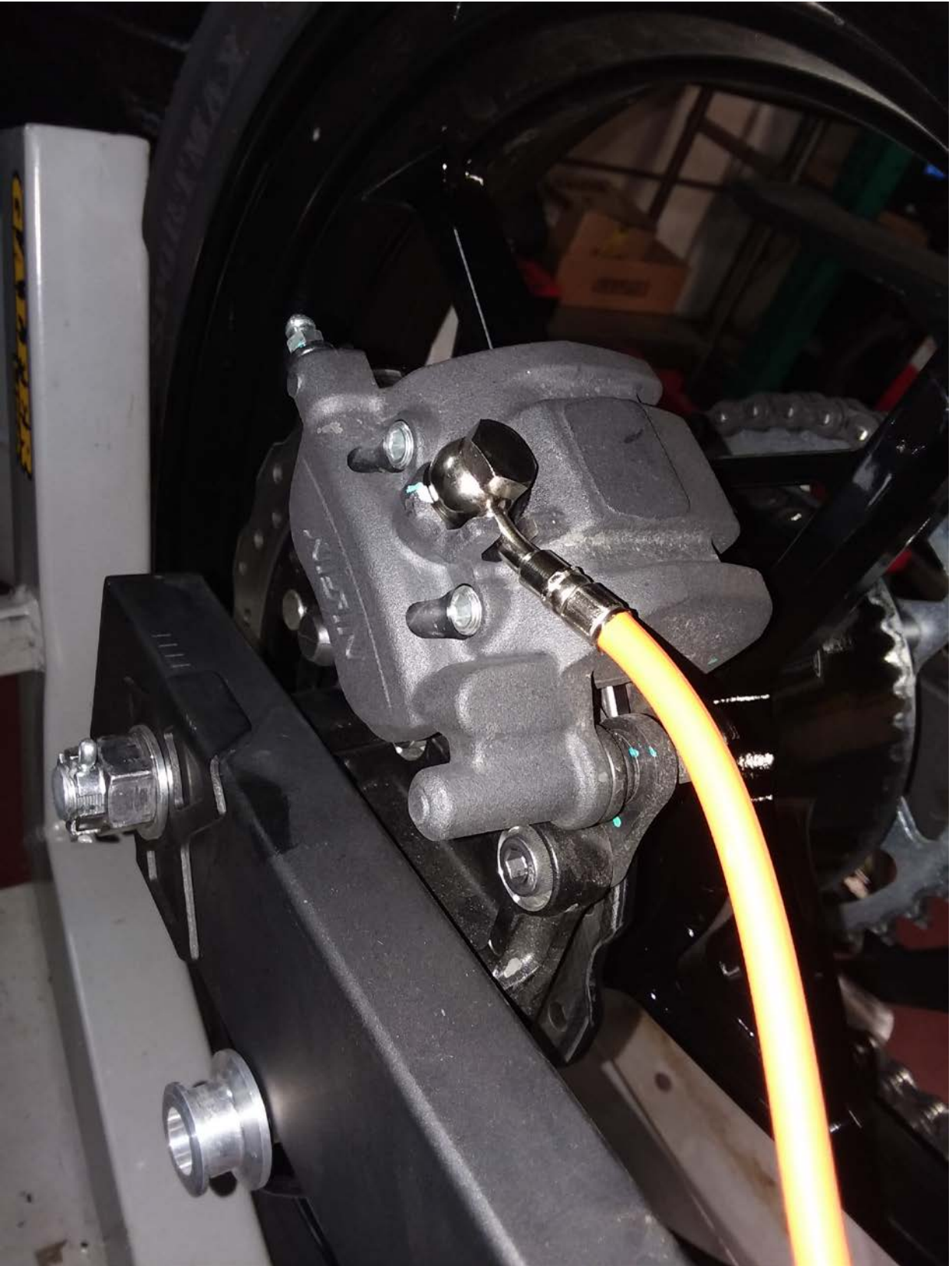
FIGURE 10: LINE INSTALLED ONTO CALIPER
