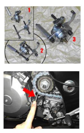
11) Place end of Cable into arm of Clutch Actuator. Bend small tab over to hold Cable end.
