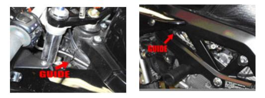
9) Remove 1 nut from end of Cable and insert threaded shaft into case mount. Place nut back on, finger tight only.
