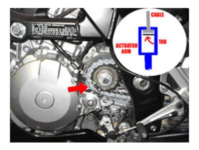
12) Install Clutch Actuator assembly. Connect spring. Note: Spring may need to be shortened to work properly.
