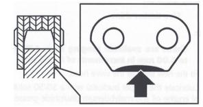
6. Check for severe wear of the plates in the area shown below.
