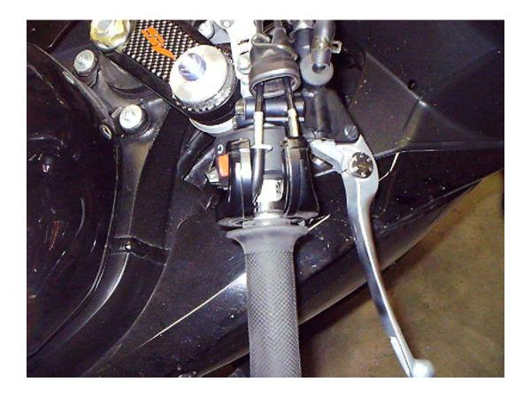
6. Remove the cables from the throttle tube, slide off throttle tube, slide on new throttle tube, and reinstall cables. Note: The holes on the tube where the cable attach will be on the bottom just like the stock one.
