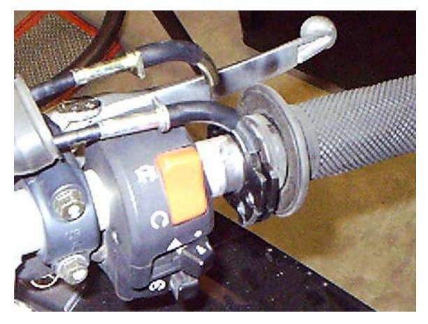
7. Reinstall the 2 halves of the throttle tube. Note: You may need to loosen the throttle cables at the adjusters to have enough slack to reinstall the throttle housing.
