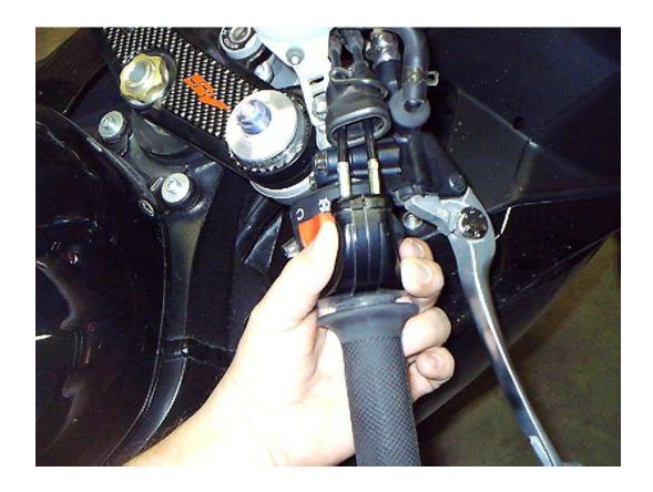
5. Carefully separate the 2 halves of the throttle housing and remove.
