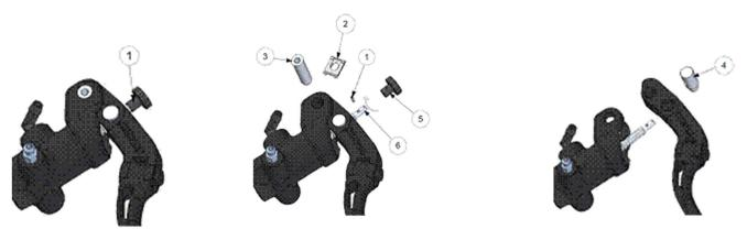
Place the master cylinder to easily remove the elastic plug, diameter 1,5mm (1) with a special pin punch. **CAREFUL**: lay the adjusting knob on a safe and stable surface, be careful not to bend the threaded pin while removing the plug.
