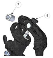
Rotate the adjusting knob clockwise (5), in order to remove the bushing (7)
