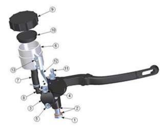
Manually screw the fluid inlet connection (1) on the new Accossato master unit.
