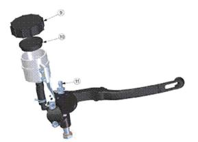
Remove the brake fluid reservoir cap (9) and the rubber seal (10).
