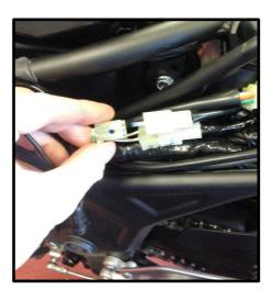
Connect the HM SR loom to crank sensor plug.
