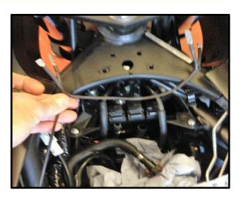
Attach the HM coil loom to the RED/BLACK wire on the coils with the spade connectors provided.
