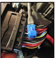
Connect the HM SR loom to the WHITE Speed sensor wire going into the ECU with the splice connector included in kit.
