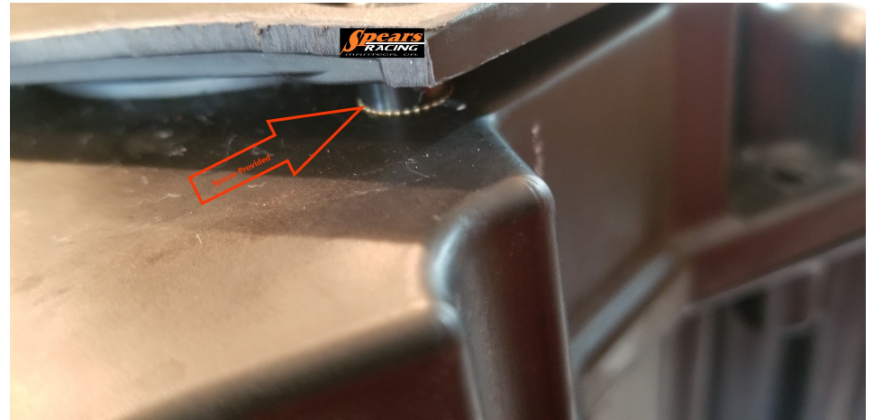
Figure 2: Spacer Installed under OEM Filter Door
