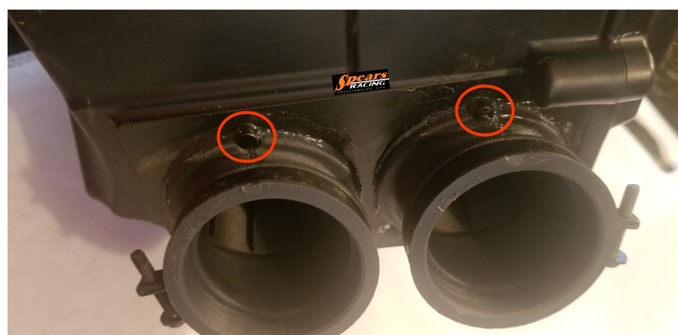
Figure 1: New manifold alignment tabs mated with the airbox alignment tabs.
