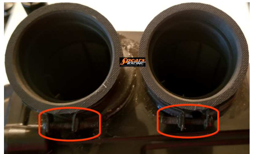
Figure 3: New manifold have no alignment tabs for the stock clamp, Install as you will
