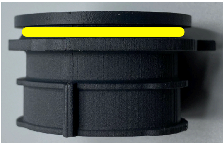
Figure 3: Location for silicone rubber sealant.
