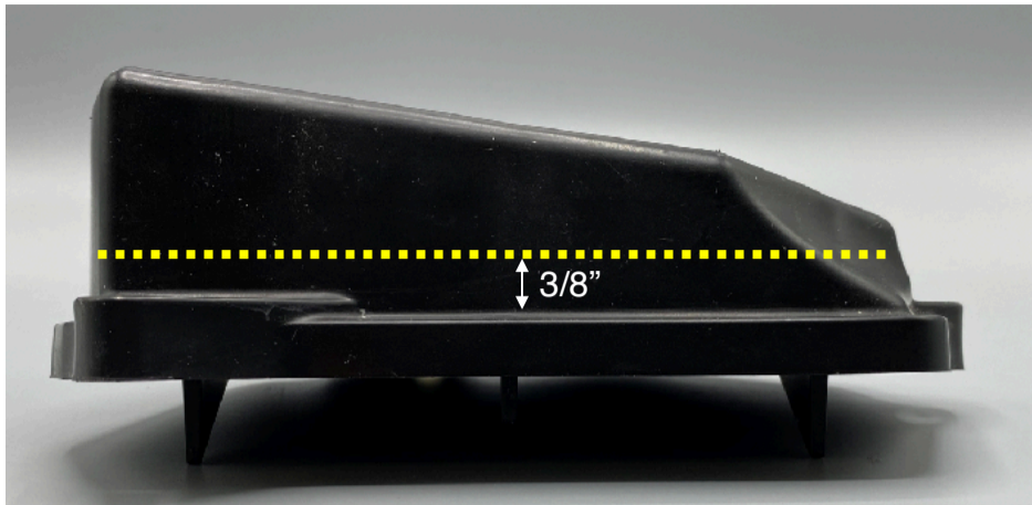
Figure 1: Air filter cover cut line.
