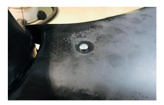
Mark, the positions for the holes, remove the tail section. Drill and tap for two (2) M8 - 1.0 screws located at the rear part of the seat (holes pre-drilled in the tail section). Screws not provided.
